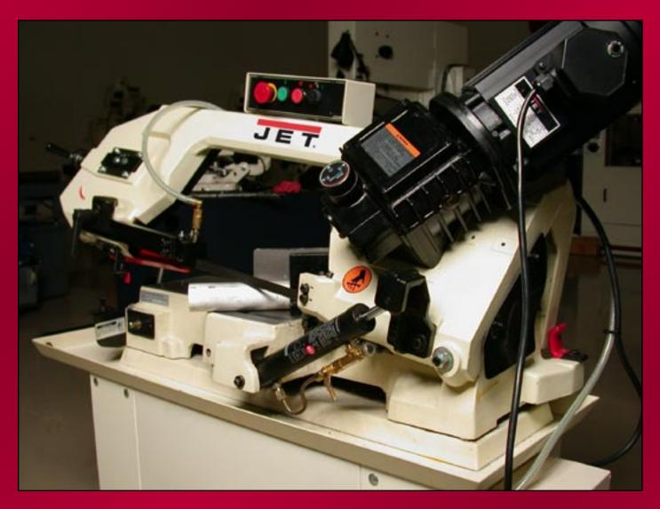
The new JET<sup>®</sup> HBS814GH horizontal bandsaw features a heavy duty gear drive to provide accurate and vibration free cutting. Featuring an 8" vertical cutting capacity, hydraulic downfeed, and enclosed coolant system. Powered by a 1 horsepower motor rated at 1720 RPM it provides three blades speeds: 135,197, 256 SFPM. Changing blade speeds is fast and easy with the turn of a dial, no belts or pulleys to replace. Mitering or straight cut-off is no problem for the HBS-814GH.
